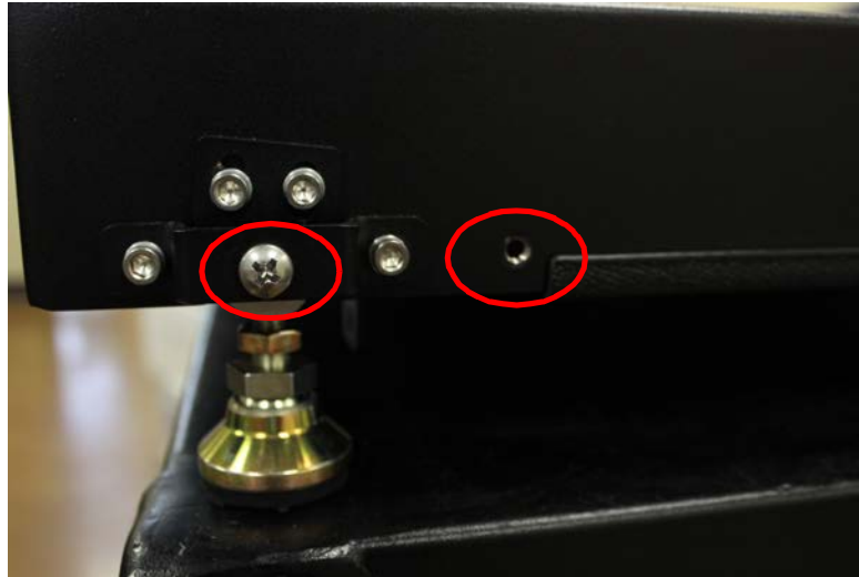
Figure 11 Shipping bolt and adjacent hole
