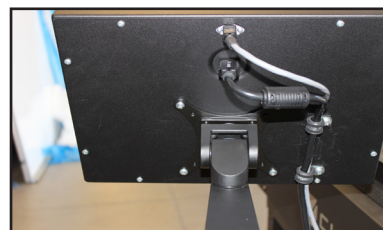
Cables plugged in and clamped.
