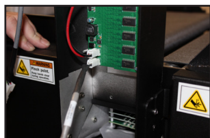
Power cable (red) and Ethernet cable connected to receptors
