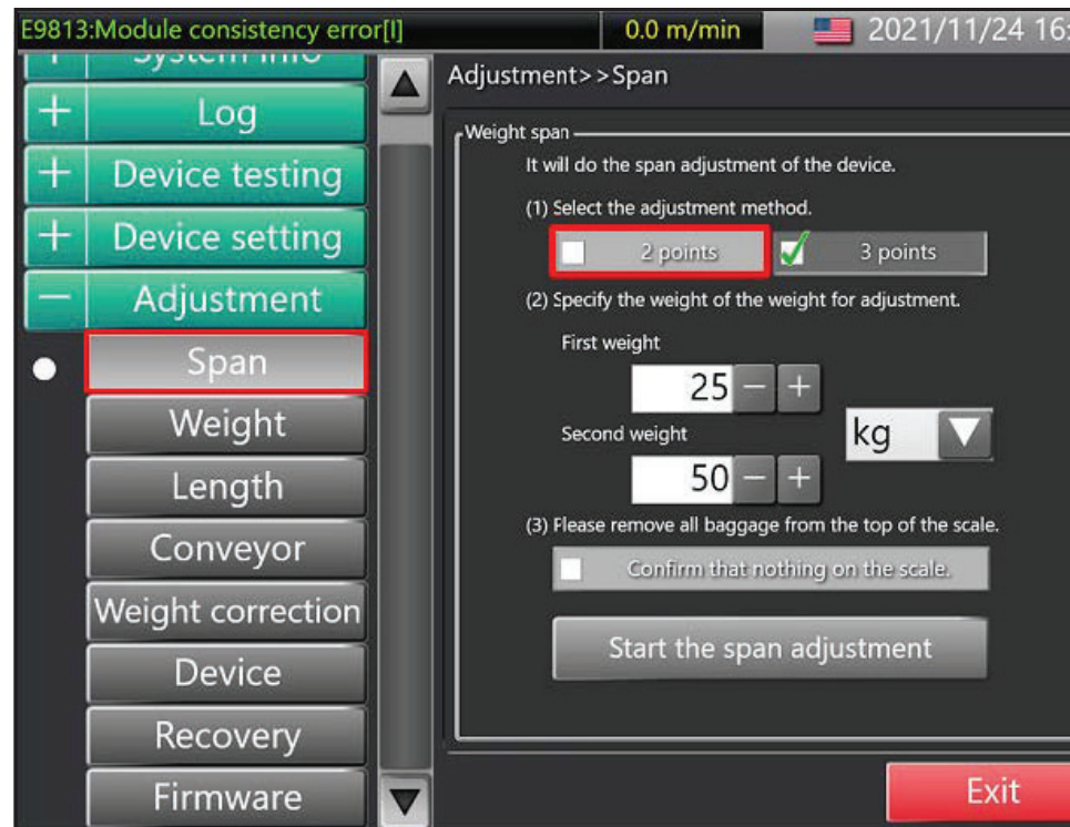
Figure 448 2-Point span adjustment - Adjustment
