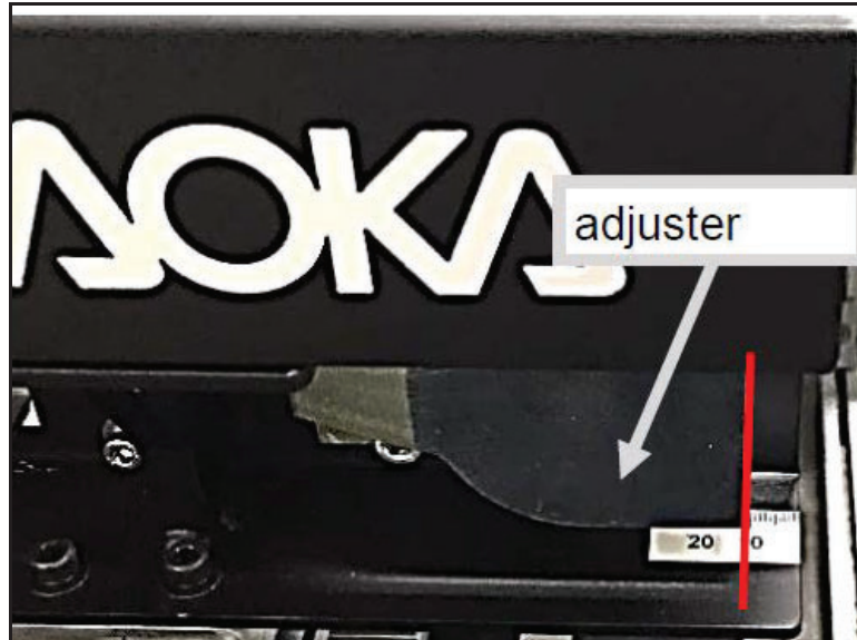
Figure 469 Reference position - B1: B conveyor front
