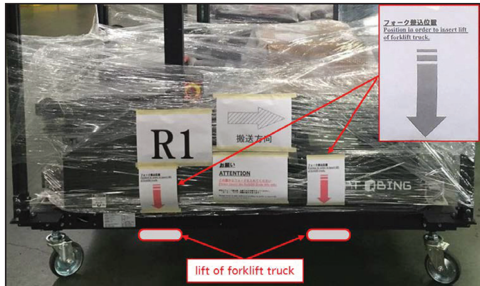
Figure 25 Unloading and installation: Designated fork holes
