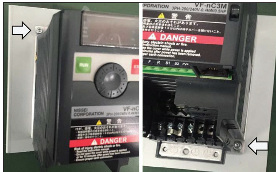
Figure 264 Inverter - Removing frame
