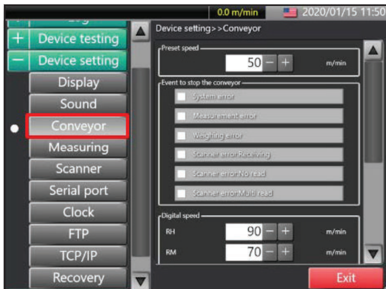
Figure 65 Conveyor setting: Conveyor screen
