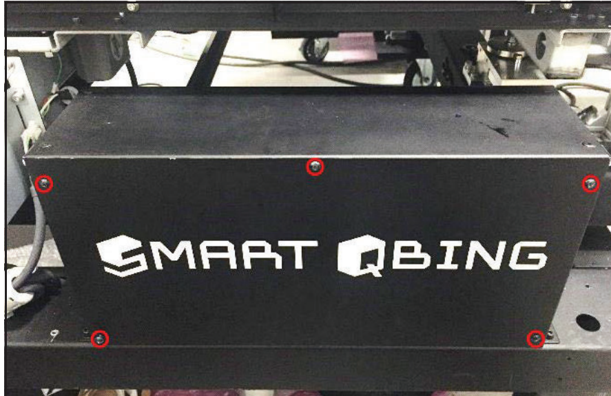
Figure 256 Inverter - Cover screws
