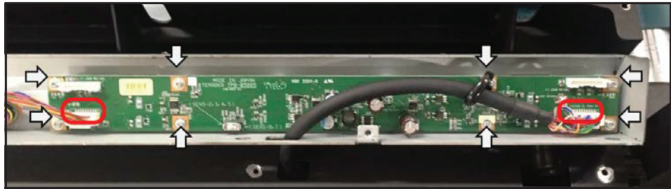
Figure 238 Conveyor B emitter - Right TPB-3865 (large) board
