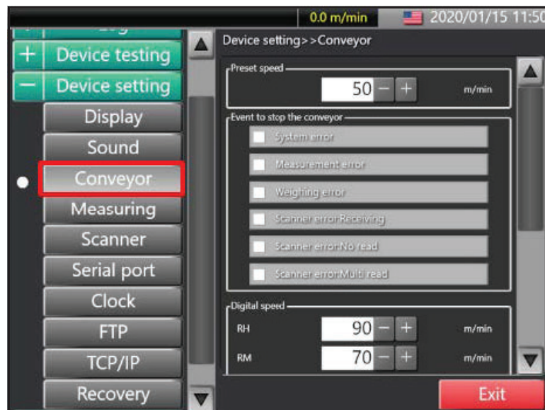
Figure 65 Conveyor setting: Conveyor screen
