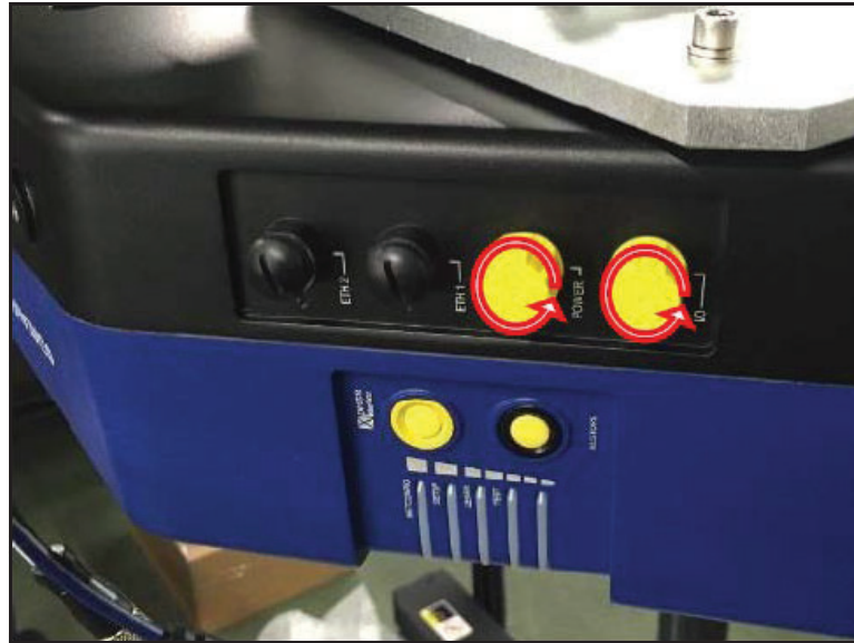
Figure 49 Fixed scanner installation: Removing connector caps
