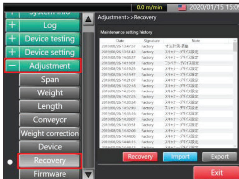
Figure 93 Setting data backup - Adjustment recovery
