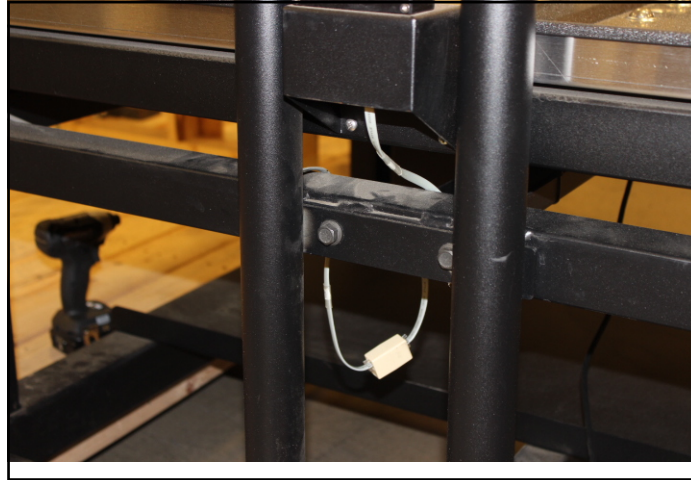
Figure 8 Height sensor cable connection
