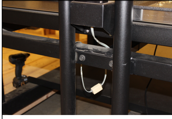
Figure 8 Height sensor cable connection
